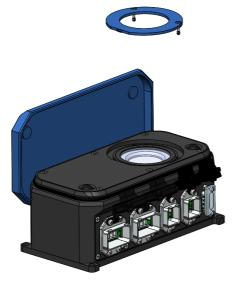
Insert the 1.5mm Allen key (or another tool) into the socket below the window with 2 pads and pick up the window from the groove.
