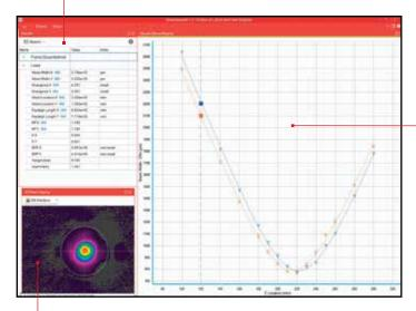
This window presents measurements of beam width vs. position for a given run. After measuring a few points, the software extrapolates a curve fit. The Xs and Ys represent individual measurement points. The solid lines present the best fit hyperbola of the beam propagation equation to the measured points. The M² and other laser parameters are computed from the best fit hyperbola since it provides a smoothing of the data points.
