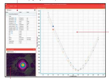
This window displays the 2D or 3D beam profile of the currently measured point in the beam propagation curve. This image enables visual intuitive verification of the beam profile behavior through focus. After each run the user can click any individual measured point and observe the beam profile. Outlying or anomalous points can be automatically or manually excluded from the curve fit calculations for more accurate results.
