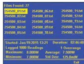
Data logs filed to USB Flash Drive. Can be viewed in StarLab or Excel.
