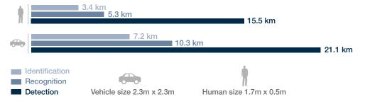
Assumptions: 32mK NETD at f/3.6 | 30Hz frame rate |  $0.2km^{-1}$  atmospheric attenuation coefficient | 50% detection probability | Johnson Criteria for DRI: Detection – 1 spatial cycles on target; Recognition – 4 spatial cycles on target; Identification – 6.4 spatial cycles on target | 1.74x0.46m,  $5^{\circ}C$  human size and  $\Delta T$  | 2.3x2.3m,  $2^{\circ}C$  vehicle size and  $\Delta T$
