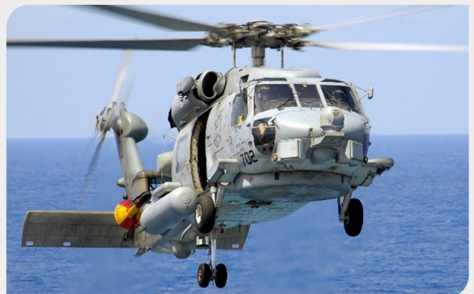
Image 2: Helicopter equipped in its front with EO system. Credit: U. S. Navy Mass Communications Specialist 3rd class James Vasquez
