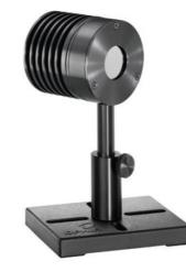
The pyroelectric sensor heat sink is designed to be fastened to the rear of PE25 and PE50 series sensors and allows the sensors to work up to higher powers without overheating. The package consists of the heat sink and a graphite thermal pad to be placed over the screw thread of the heat sink when it is fastened to the sensor so as to make good thermal contact between the sensor and the heat sink.
