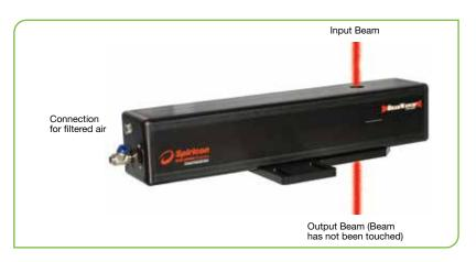
BeamWatch utilizes disruptive technology to measure laser beam characteristics of very high power lasers. By not intercepting the beam and yet providing instantaneous measurements, you can now monitor the beam at frequent intervals without having to shut down the process or remove tooling and fixtures to get access. In addition, you can now measure focal spot location at several times per second and know if there is any focal spot shift during those critical start-up moments.
