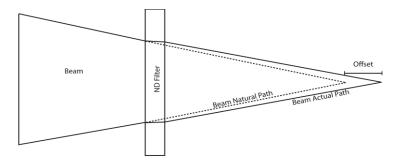
Each beam splitter housing and ND Filter holder has its own calibrated dimensions printed and placed on the unit. To calculate the total path length, we need to look at all the variables.
