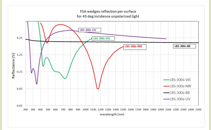
Reflectance Spectra demonstrates single surface reflection. The combined reflection of wedges is a multiplication of the percentage value of a single surface.
